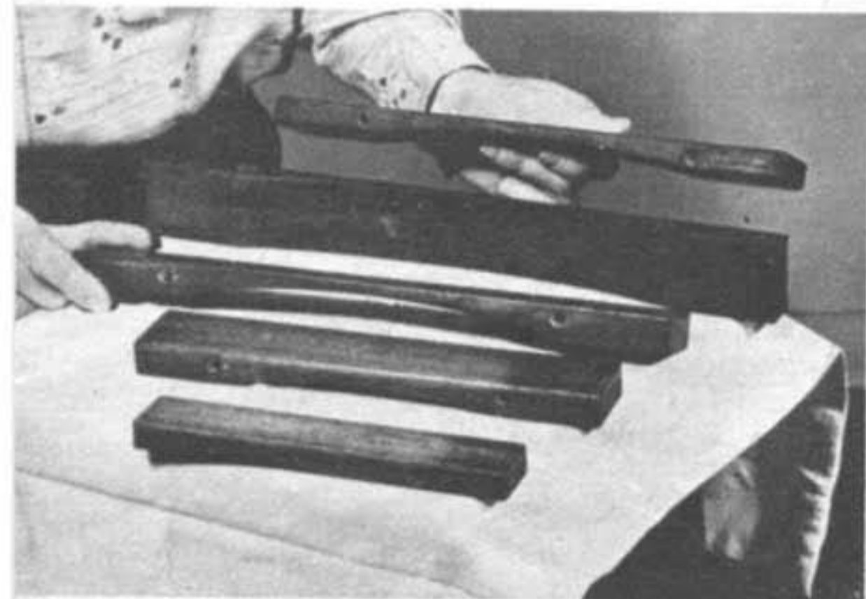
Concave undersides of keys. Center thickness is one factor which determines pitch.
