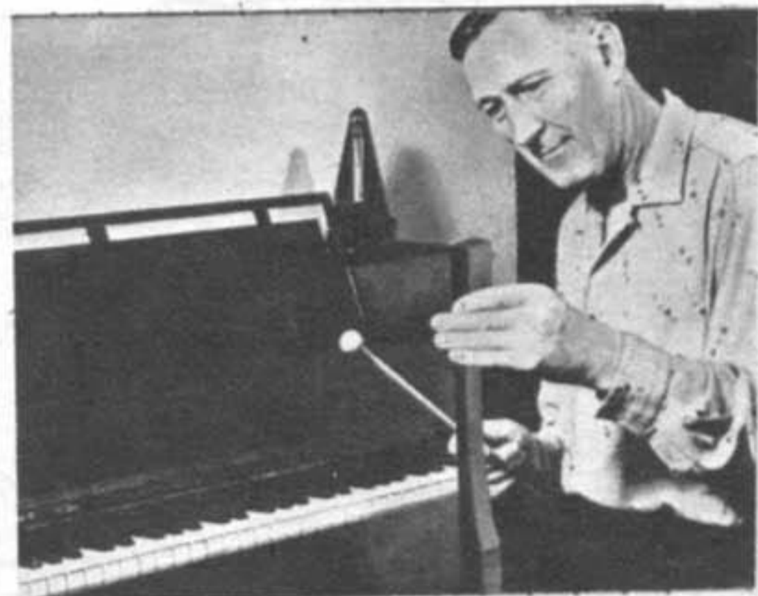
Key is held at node and pitch is compared with that of corresponding key on a piano.
